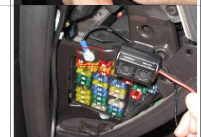
Attach the Ground wire (Black) of the Direct Power Module to the bolt at the top of the fuse panel. Make sure the spade on the end of the wire makes good contact with the metal on the bolt head.
