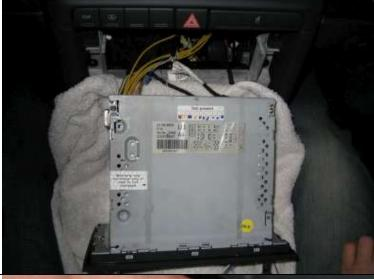
Pull the head unit out onto the towel and pull the edges of the towel up into the cavity to prevent scratching.
