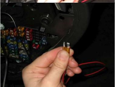
Fold the exposed wires over the right side of the tip of the 5A fuse that corresponds to fuse 16 for the Garage Door Opener.
