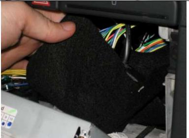
Wrap the ADR interface box with some felt or something to prevent rattling to prepare to stuff it in the open space behind the head unit once it is reinstalled.
