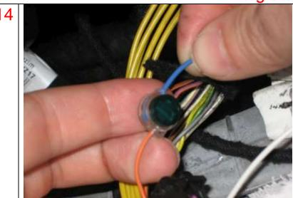
Place the ends of the ADR harness into the corresponding wires.
