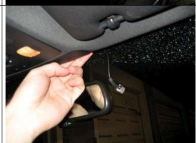
Take the V1 back out and start placing the cable. Hold the cable with one hand while using our trim wedge to stuff cable in the space between the windshield and the headliner.
