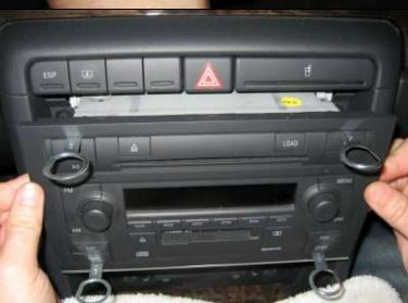
Use the Radio Removal Tools in the 4 slots in the radio's face to remove the head unit.
