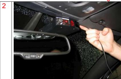
Place the V1 and plug it in to make sure you leave enough slack to plug the V1 in after routing the cable.
