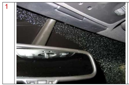
Clean off the area where are you are planning on placing the V1. Most people put it on the passenger side of the rear view mirror on the windshield. This allows for an easy route for the cables to get under the dash by going around where the windshield and the headliner meet.
