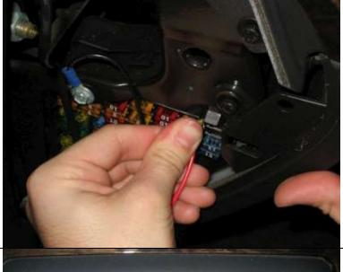
Plug the fuse with the wires into the jack. You shouldn't have to force it. If it is too hard to plug in, cut some more of the exposed wires away and try it again.
